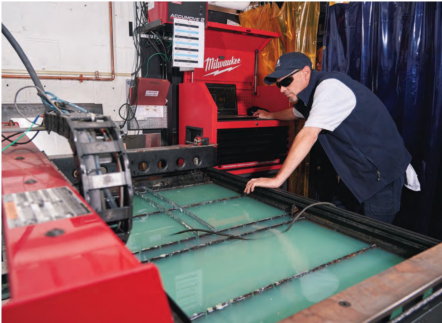
George Calloway works the plasma cutter, which only requires one person to operate
